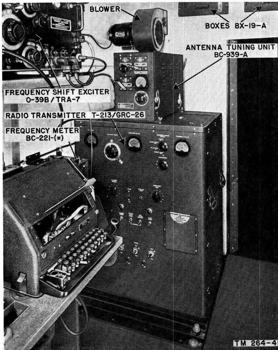
Figure 4. Radio Set AN/GRC-26, transmitting components.
