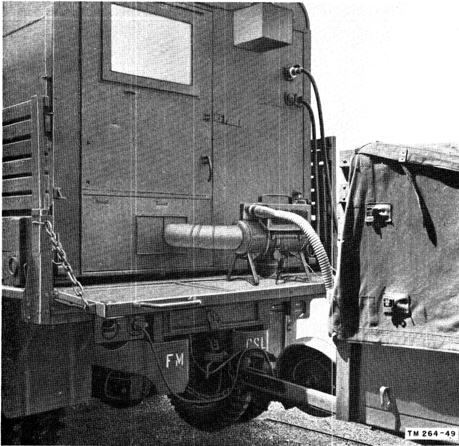
Figure 46. Gasoline Heater OG-31 in use.
